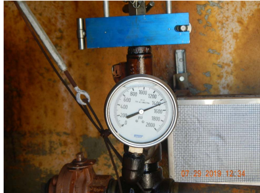
Photo 2. Tubing pressure at time of inspection.
