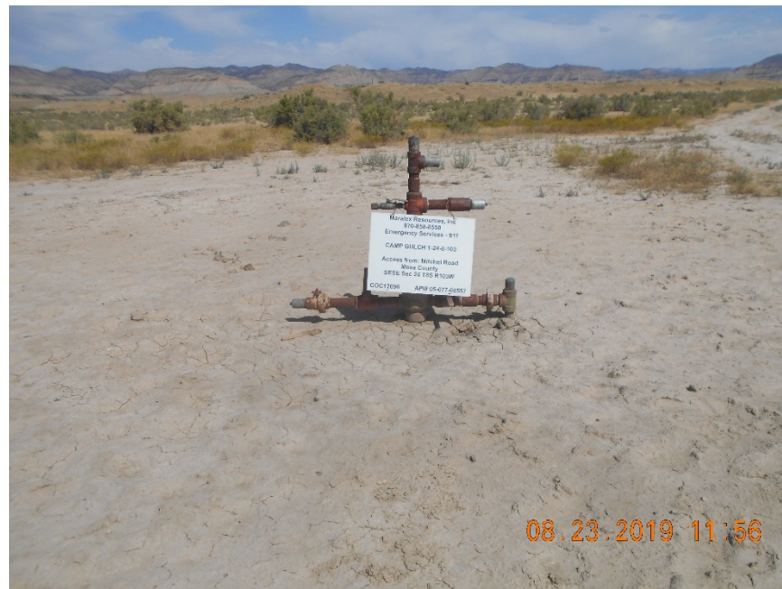
Wellhead with sign - Temporarily Abandoned.
