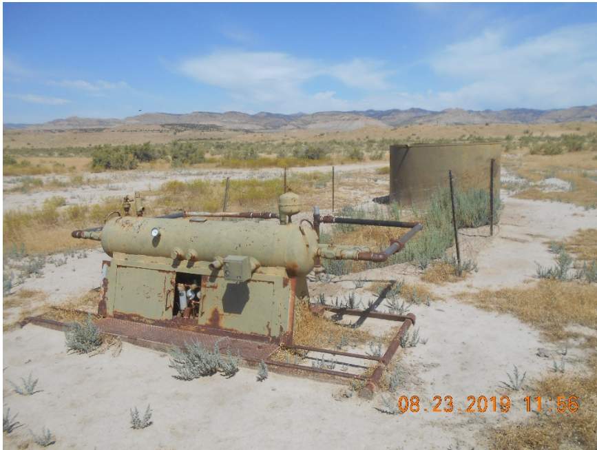
Separator with blowdown pit.
