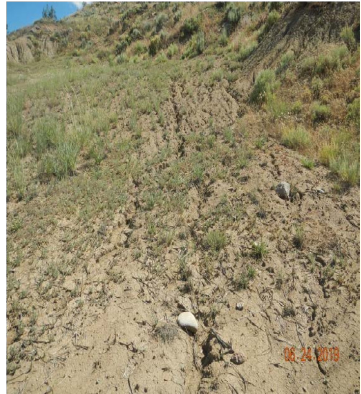
Photo#9: Erosion where erosion blanket not installed.
