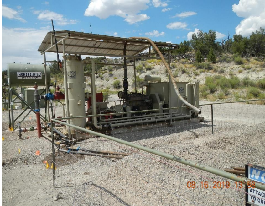
Stained and wet gravel beneath hammer unions on flow lines.
