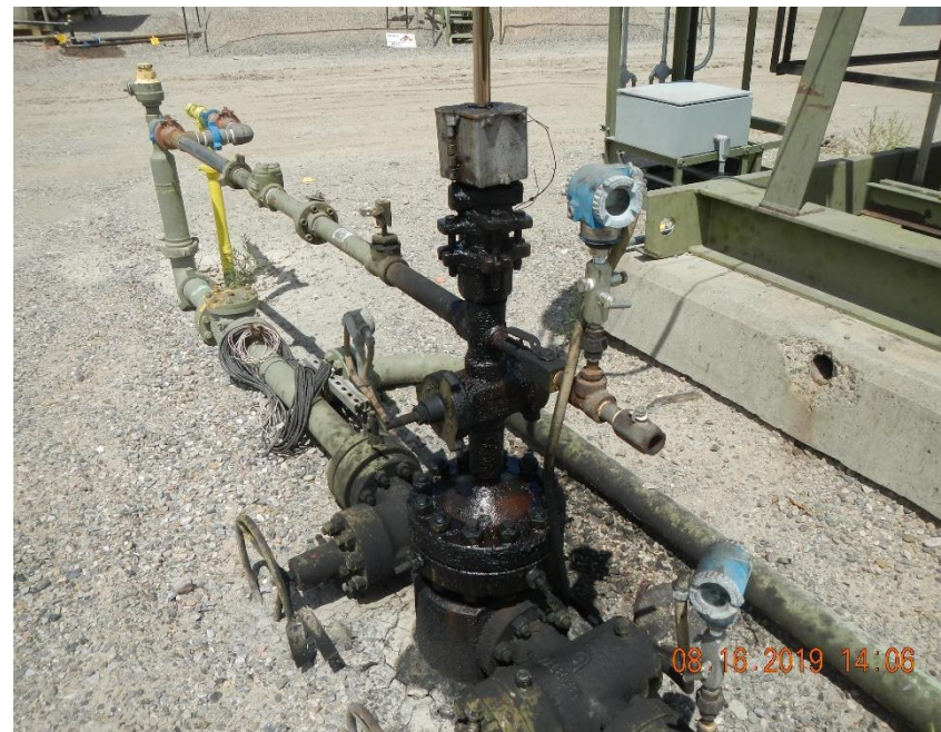
Well head is stained and wet.
