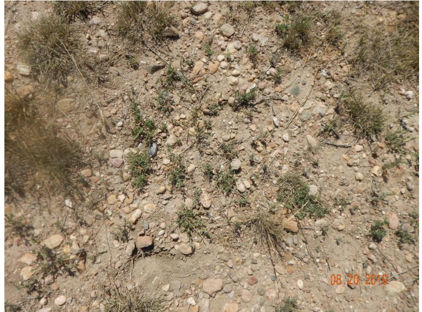
Photo 4: Photo shows gravel/road base remaining on location appears to be hindering reclamation.
