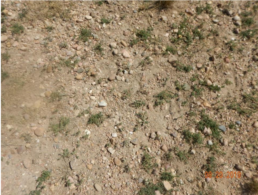
Photo 5: Photo shows gravel/road base remaining on location appears to be hindering reclamation.
