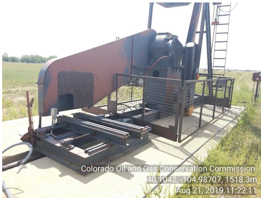
Photo 3 Missing Electric Motor & Belts laying on ground
