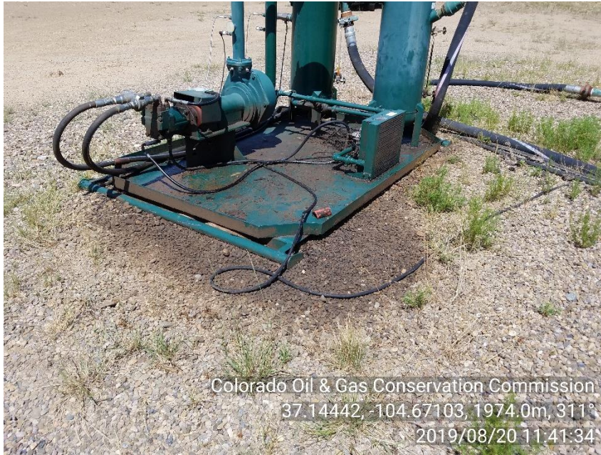
PHOTO 3: AREA OF IMPACTED SOIL NEAR COMPRESSOR. Remove and dispose impacted material in approved manner, service and maintain equipment and self inspect to prevent recurrence of conditions per 1002.f(2) and 907. CA DATE 9/20/19.
