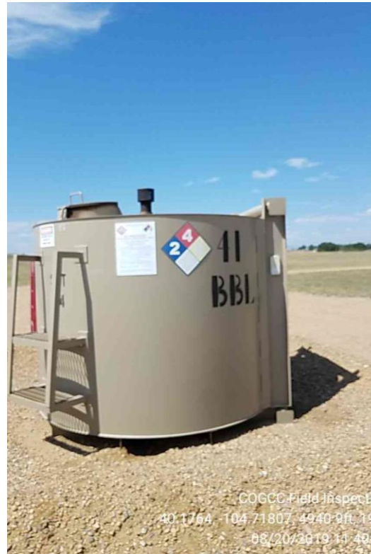
Photo 2 Bradenhead Collection Tank
