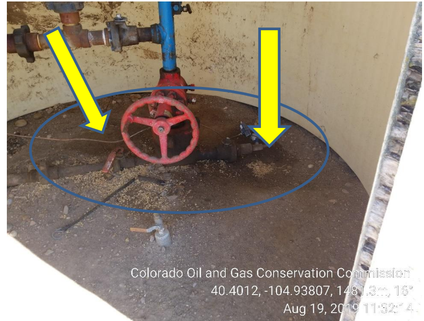
Photo 4: Stained soil at wellhead
