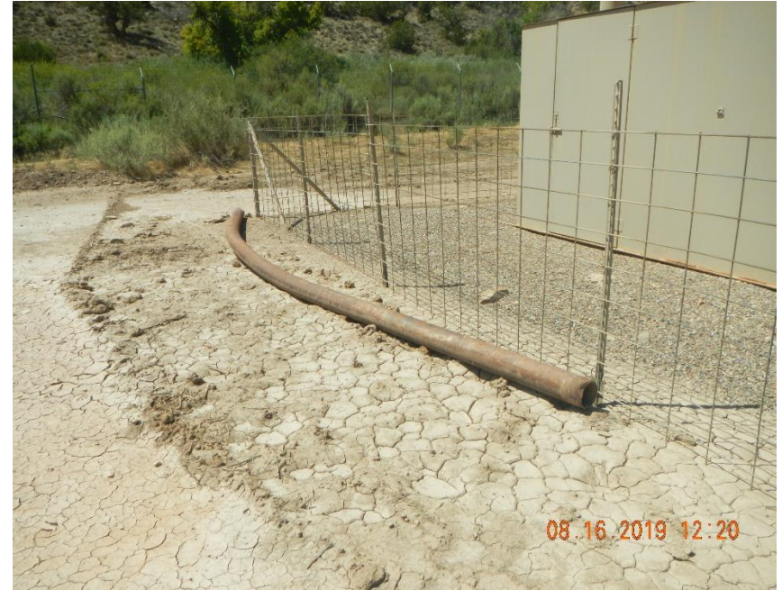
Unused equipment. Piece of 4" casing at separator fence.
