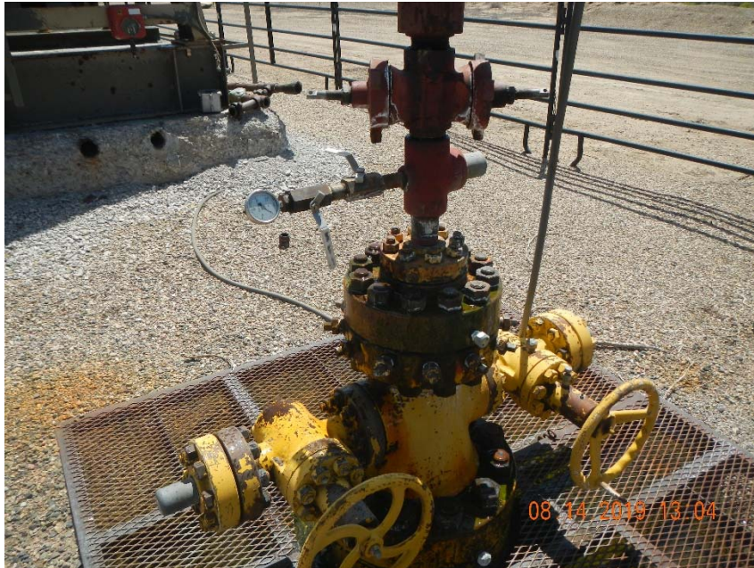
Photo 1. Ongoing leak occurring at wellhead.
