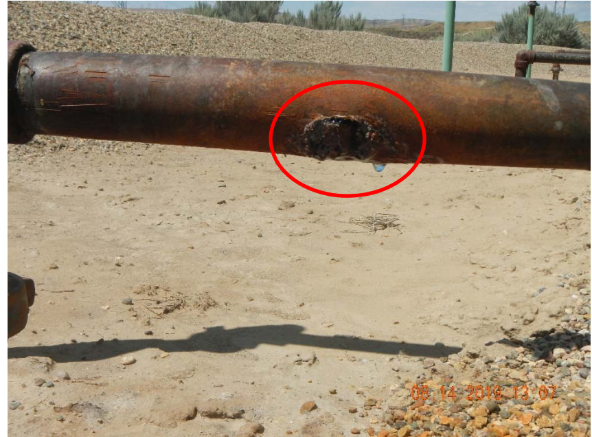
Photo 4. Close up of photo 3, leaking area circled in red.
