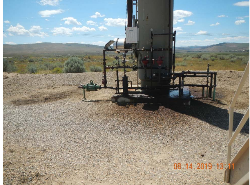
Photo 6. Stained soil and free fluid at separator.
