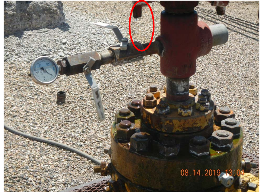
Photo 2. Close up of photo 1, leaking area circled in red.
