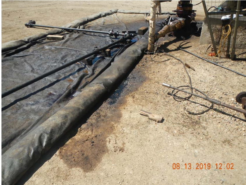
Photo 3. Non reportable spill at wellhead. Containment that has become trash/debris at wellhead.
