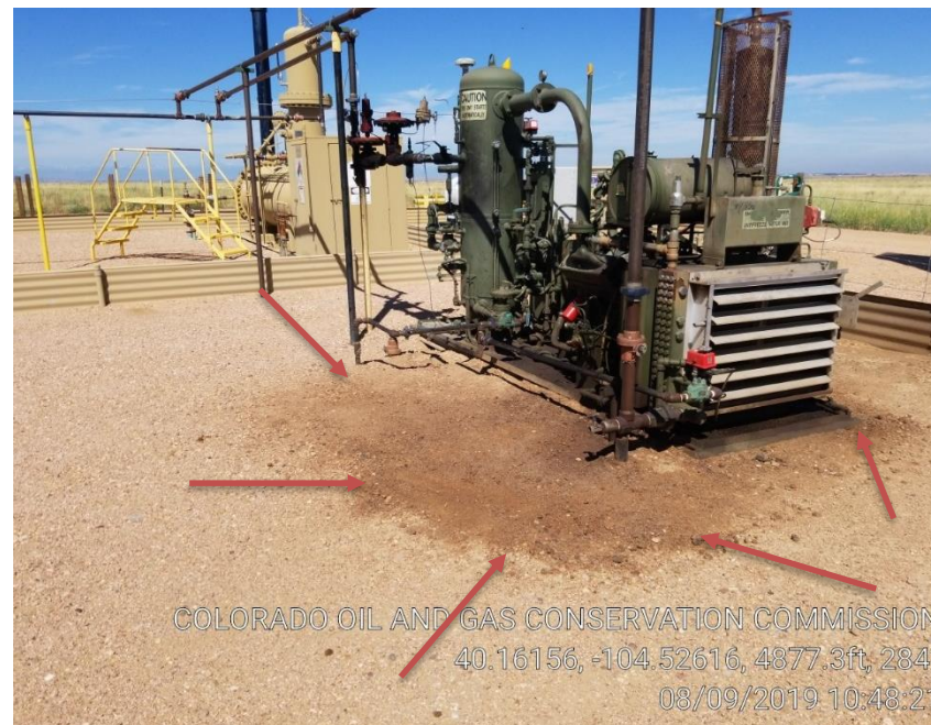
Pic 8 stained soil/mechanical issues
