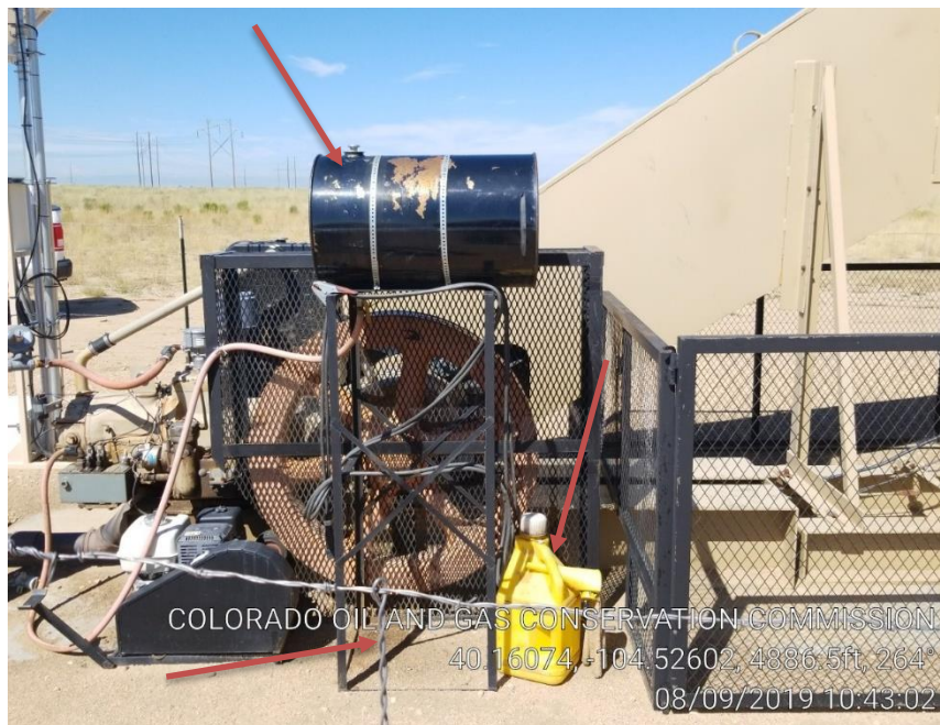
Pic 3 stained soil & no containment for chemicals
