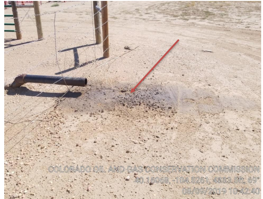
Pic 2 stained soil by muffler of pumping unit.
