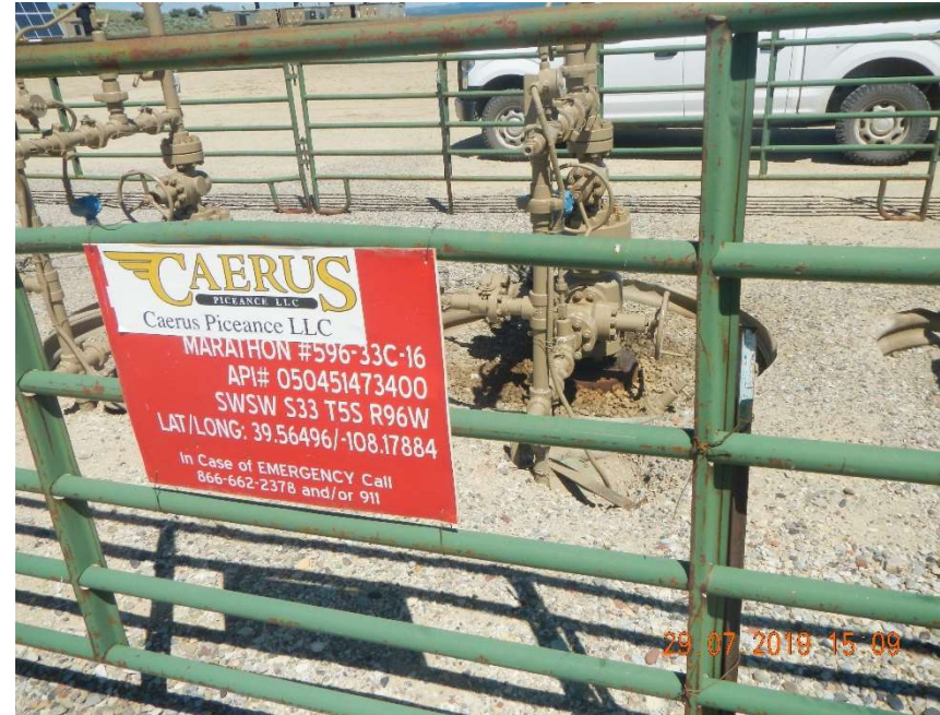
Photo #4 - Localized accumulation of oily waste (oil-stained soil) in the 596-33C-16 cellar.
