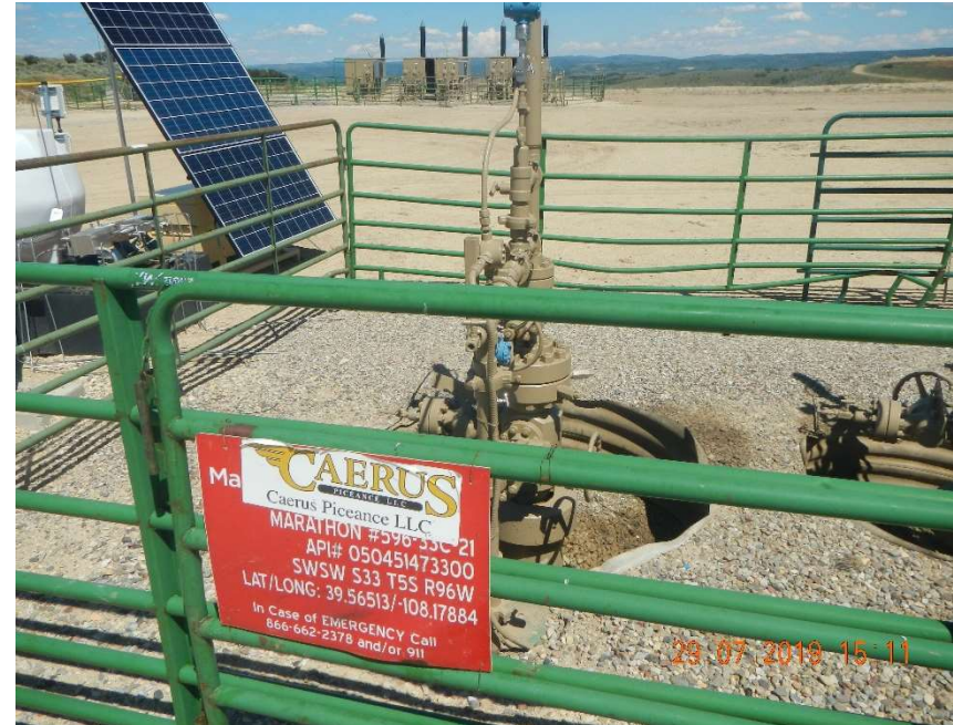
Photo #6 - - Localized accumulation of oily waste (oil-stained soil) in the 596-33C-21 cellar. Uncovered cellars with no wildlife egress.
