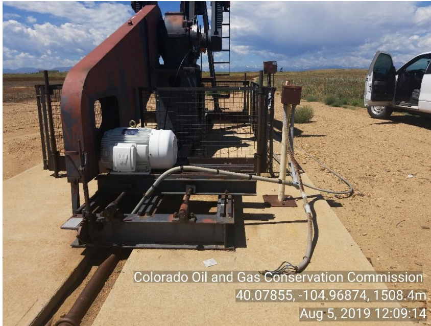
Loc photo 3 Mech issue Exposed wiring
