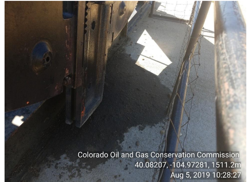
Photo 6 Stained soil under gear box
