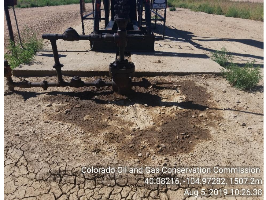
Photo 2 Stained soil around WH
