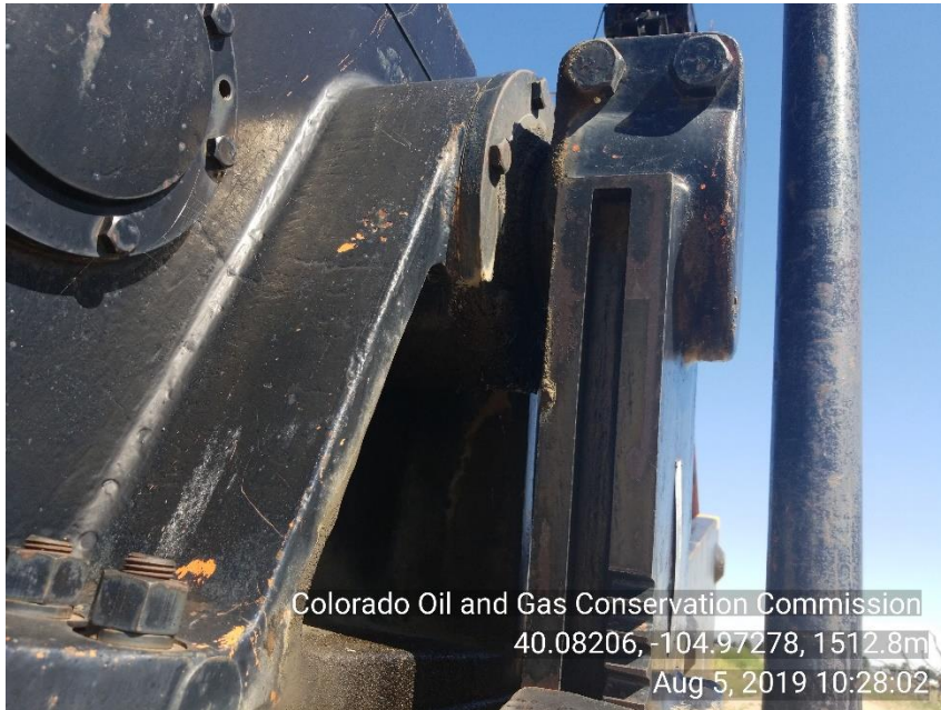
Photo 5 Mechanical issue Gear box bearing appears to be leaking
