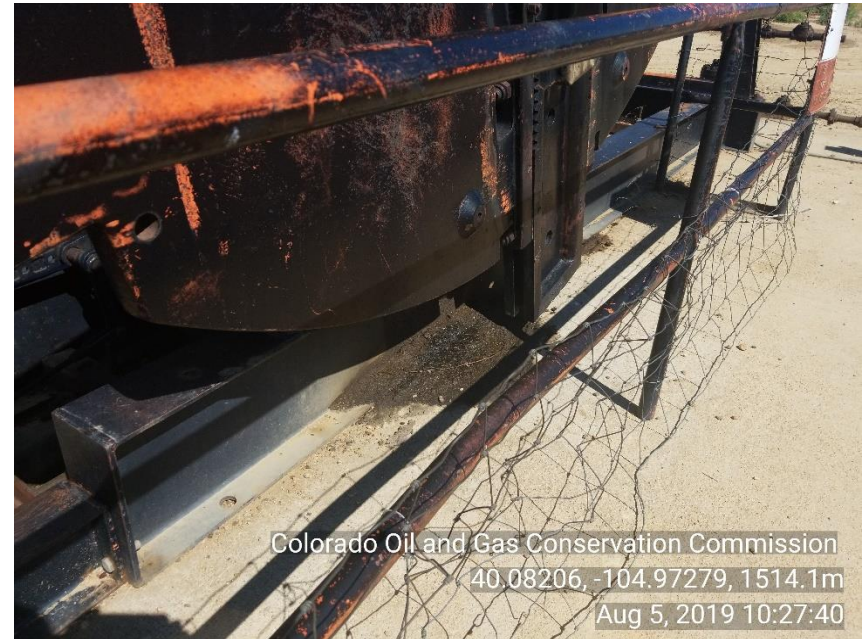
Photo 4 Stained soil under gear box
