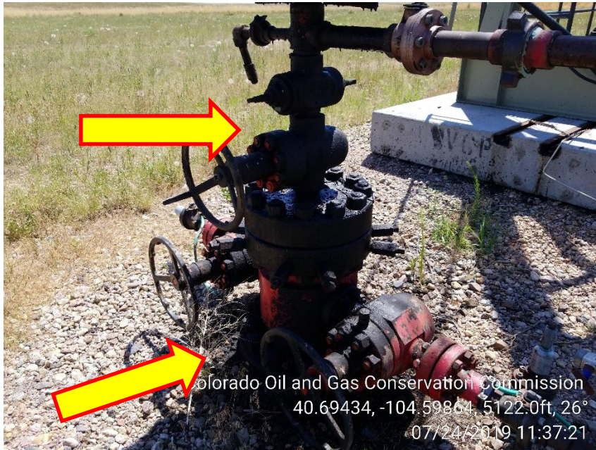
Photo 3 – Wellhead appears to be leaking. Stained Soil
