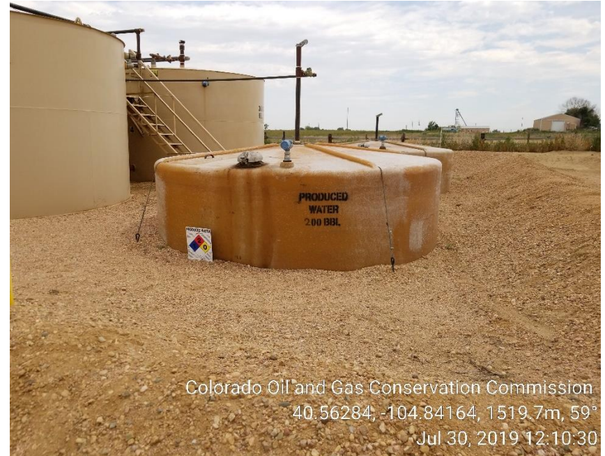
Photo 2: Labeling on produced water tank added
