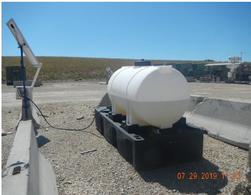
Chemical container at wells is missing label.
