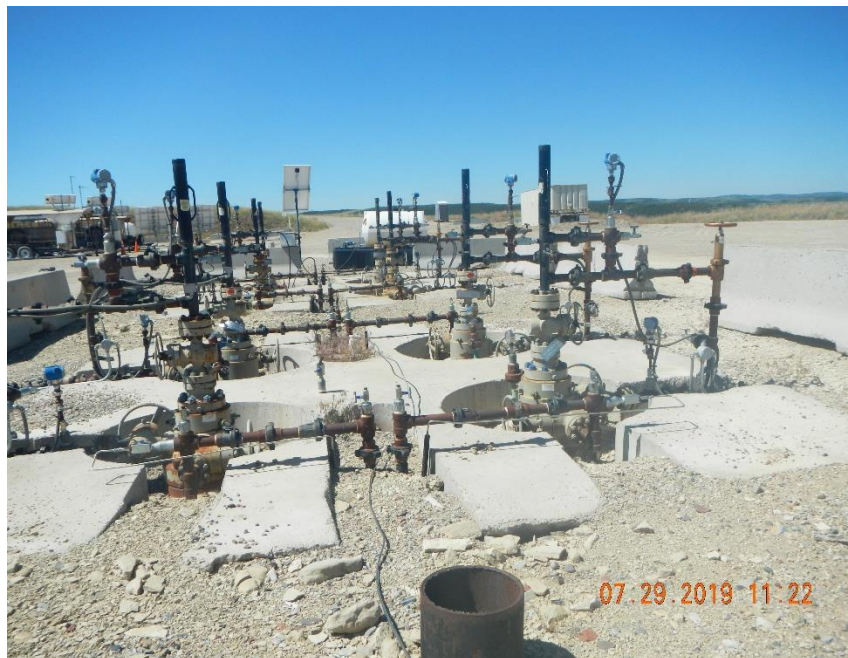
An open casing between the 2nd and 3rd quadrant of wells.
