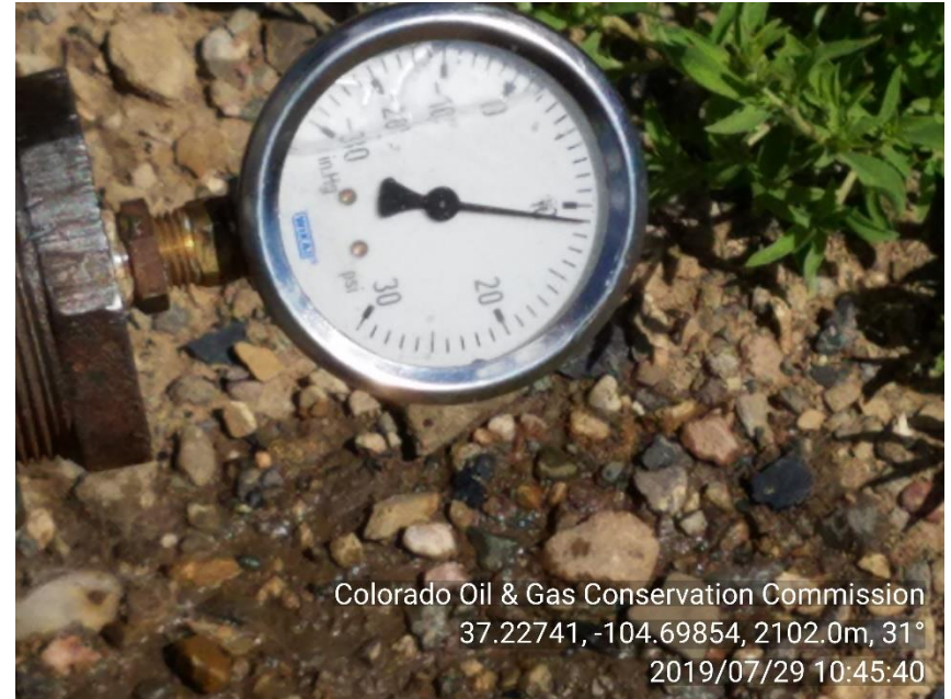
PHOTO 4: 11 PSI ON BACKSIDE BETWEEN TBG & CSG. MONITORED PSI FOR 15 MIN. NO CHANGE.
