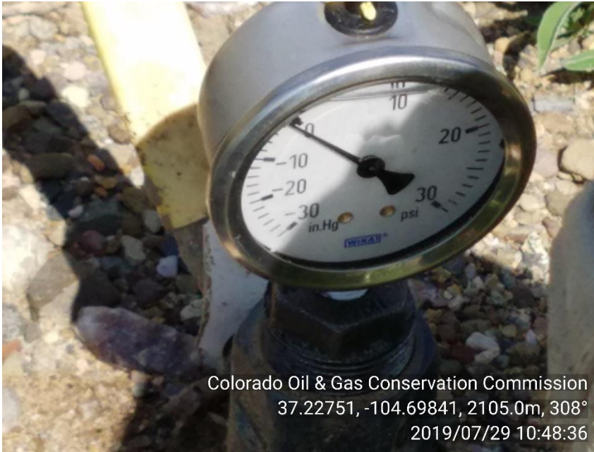
PHOTO 5: 0 PSI ON BRADENHEAD. MONITORED FOR FLOW FOR 15 MIN. NO FLOW.
