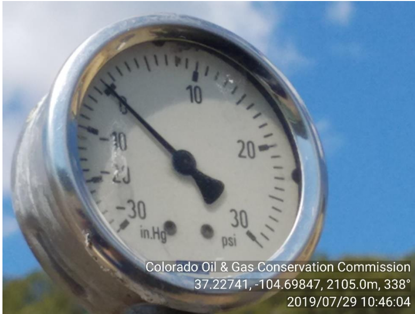
PHOTO 3: 0 INJECTION PSI WELL IS SI
