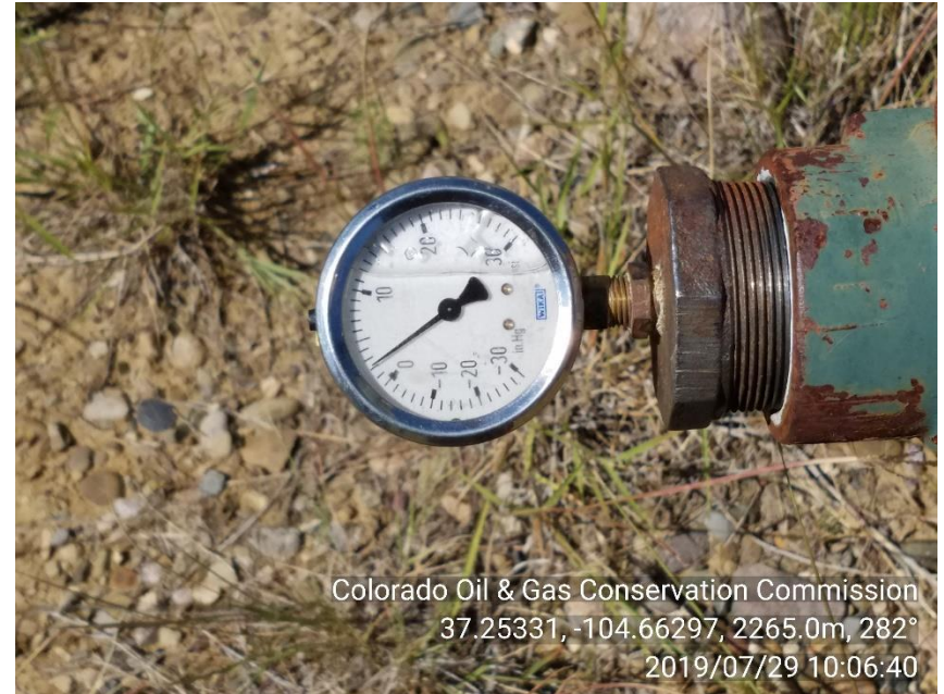
PHOTO 4: 3 PSI ON BACKSIDE BETWEEN TBG AND CSG. MONITORED FOR 15 MIN. NO CHANGE.
