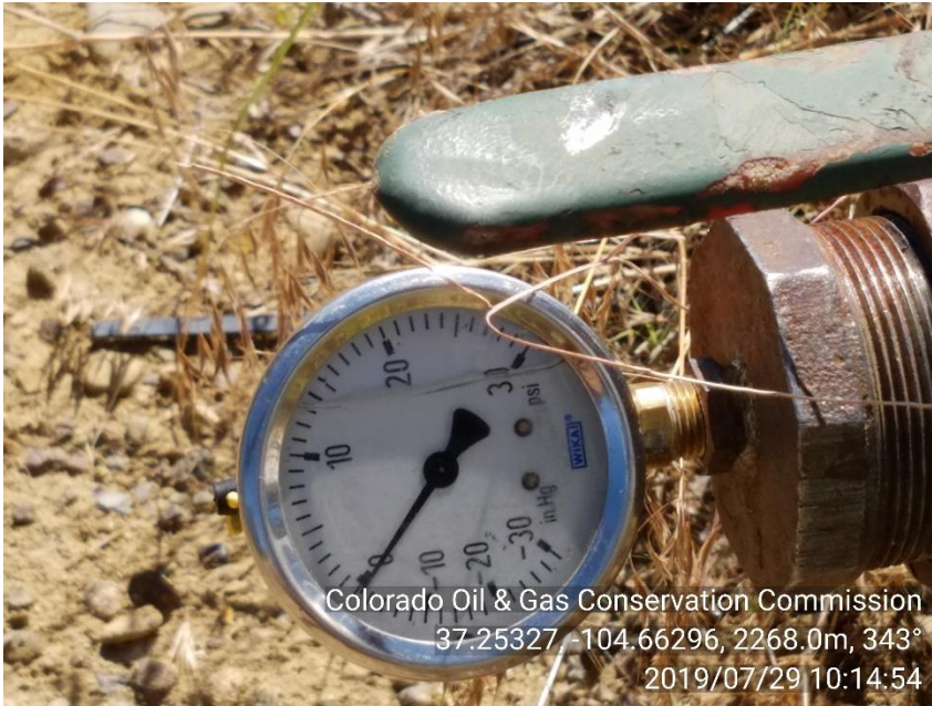
PHOTO 5: 0 PSI ON BRADENHEAD. MONITORED FOR FLOW 15 MIN. NO FLOW.
