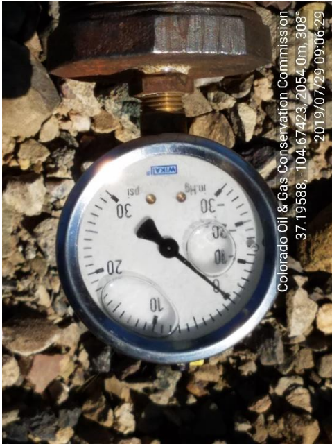
PHOTO 5: BRADENHEAD 0 PSI MONITORED FOR FLOW 15 MIN. NO FLOW.
