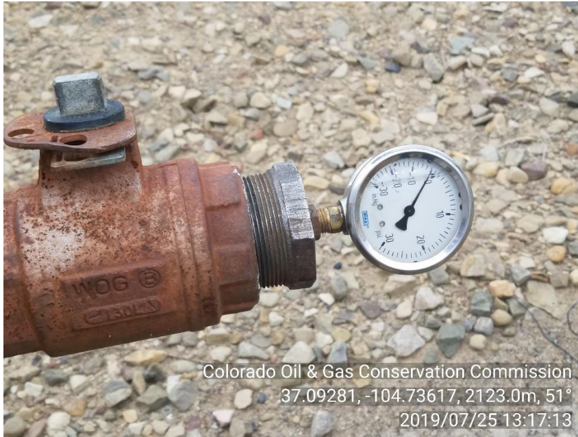
PHOTO 5: BACKSIDE BETWEEN TBG & CSG O PSI MONITORED FOR 15 MIN. NO GANGE
