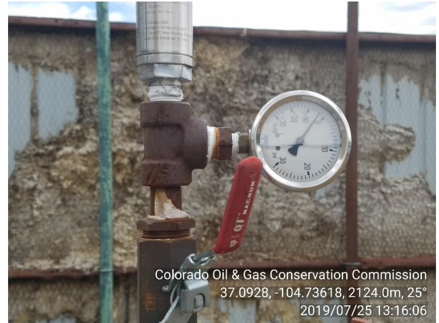
PHOTO 4: INJECTION -4 PSI MONITORED FOR 15 MIN. NO CHANGE
