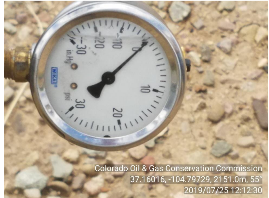
PHOTO 4: BACKSIDE BETWEEN TBG & CSG 0 PSI MONITORED FOR 15 MIN. NO CHANGE
