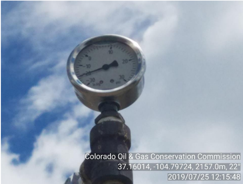
PHOTO 3: INJECTION -20 PSI MONITORED FOR 15 MIN. NO CHANGE
