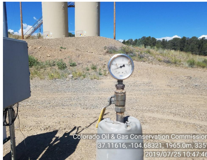
PHOTO 2: INJECTION -21 PSI MONITORED FOR 15 MIN. NO CHANGE
