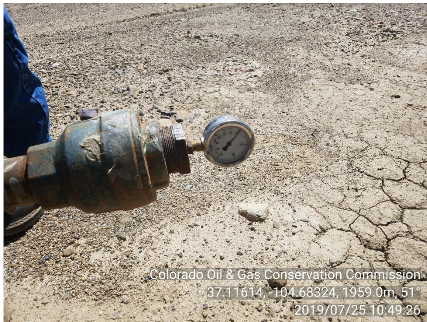
PHOTO 3: PSI BETWEEN TBG & CSG 0 PSI. MONITORED FOR 15 MIN. DO CHANGE
