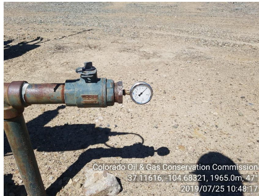
PHOTO 2: BRADENHEAD 0 PSI MONITORED FLOW FOR 15 MIN. NO FLOW
