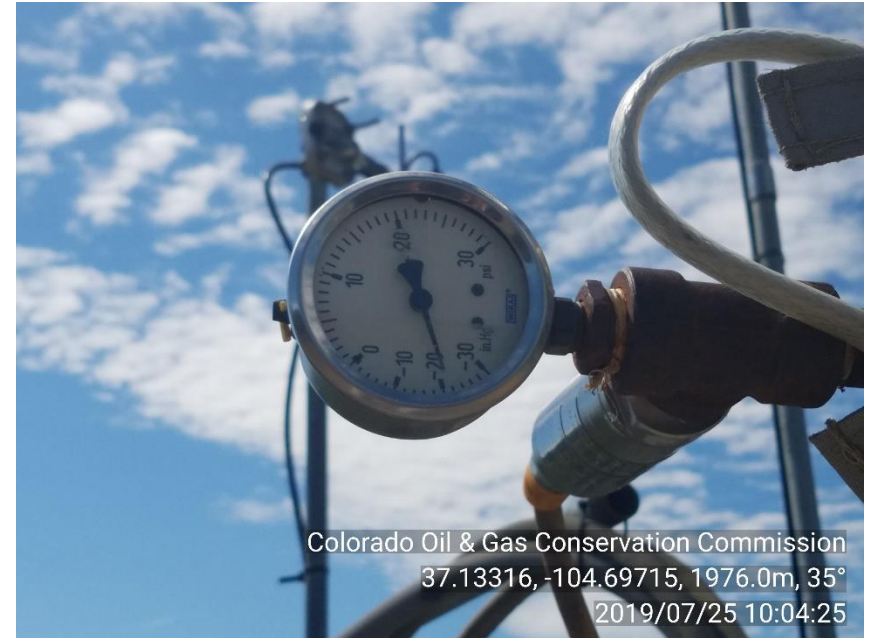
PHOTO 4: INJECTION PRESSURE -21 PSI NO FLUCTUATION
