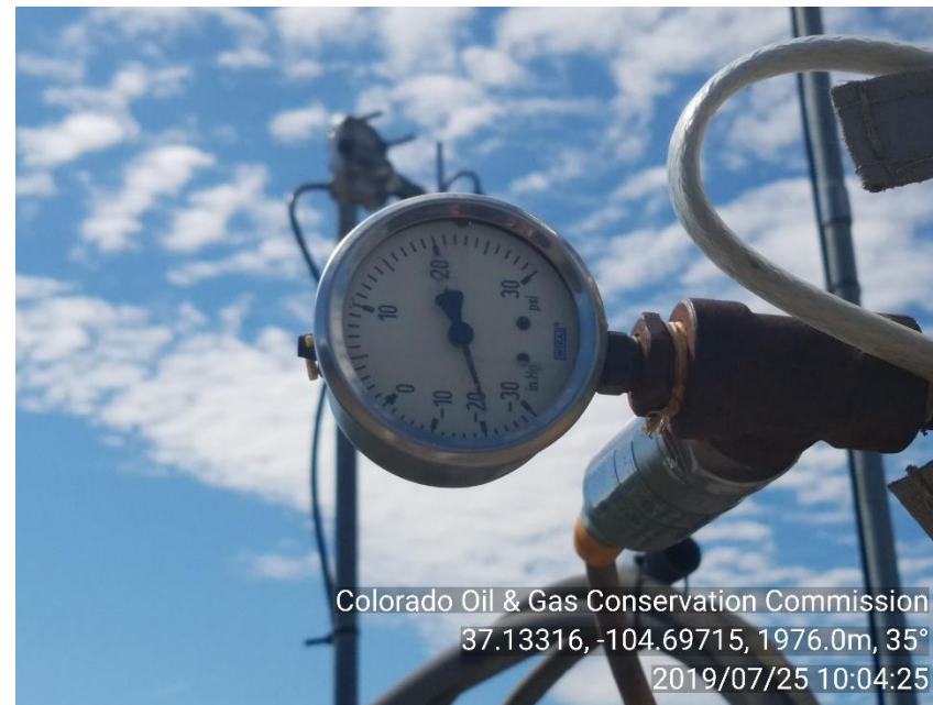
PHOTO 4: INJECTION PRESSURE -21 PSI NO FLUCTUATION FOR 15 MINUTES.
