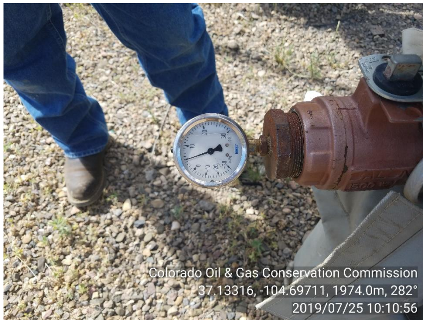
PHOTO 5: BETWEEN TBG & CSG 5 PSI NO FLUCTUATION FOR 15 MINUTES.
