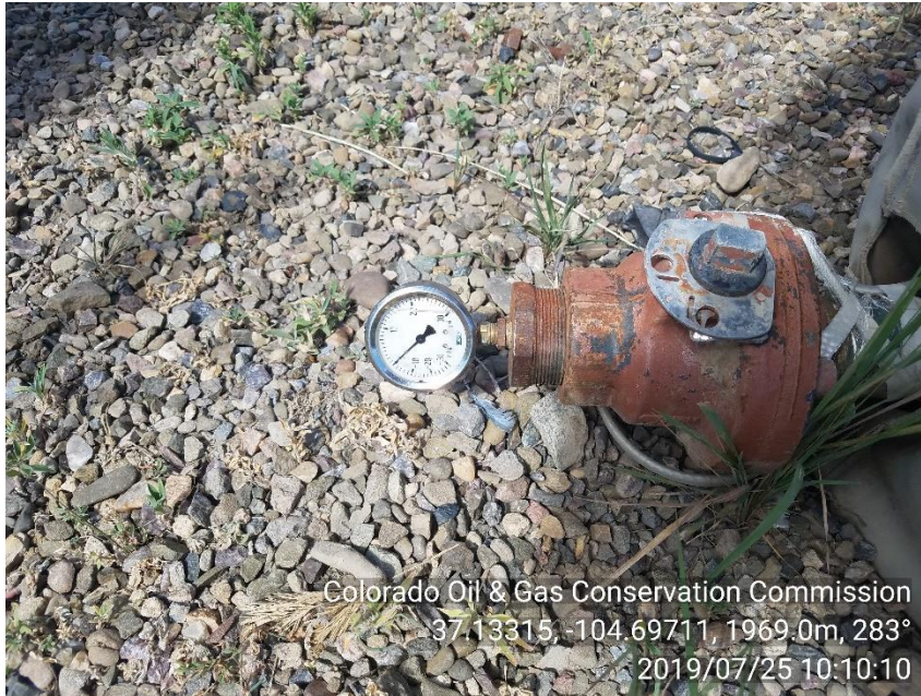
PHOTO 5: BRADENHEAD 0 PSI NO FLOW FOR 15 MINUTES.
