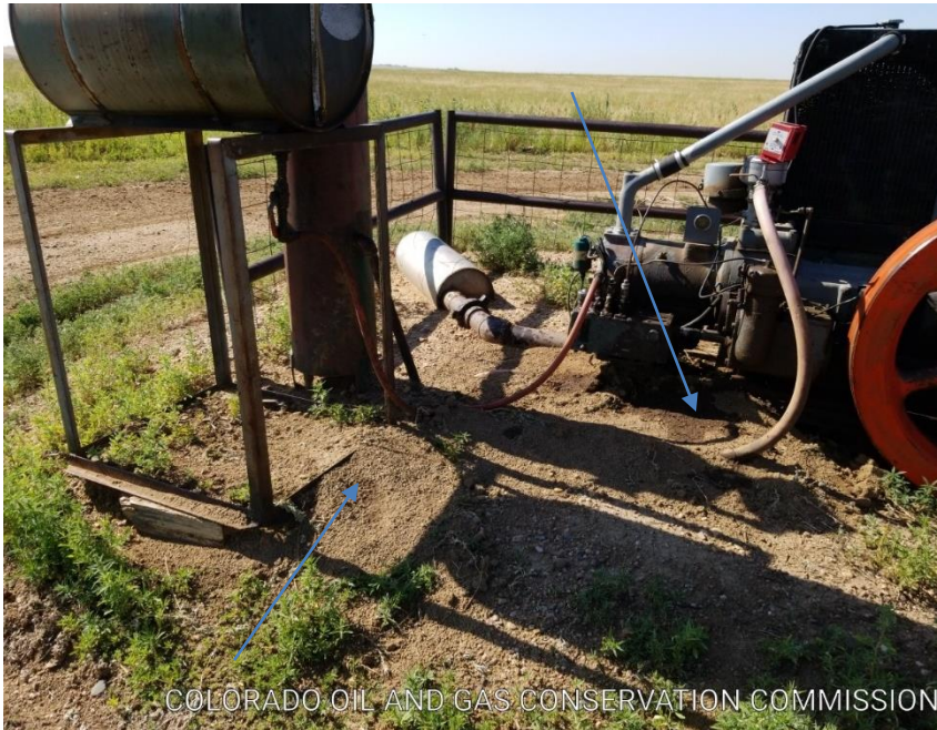
Pic 3 stained soil by motor, no BMP for chemical tank
