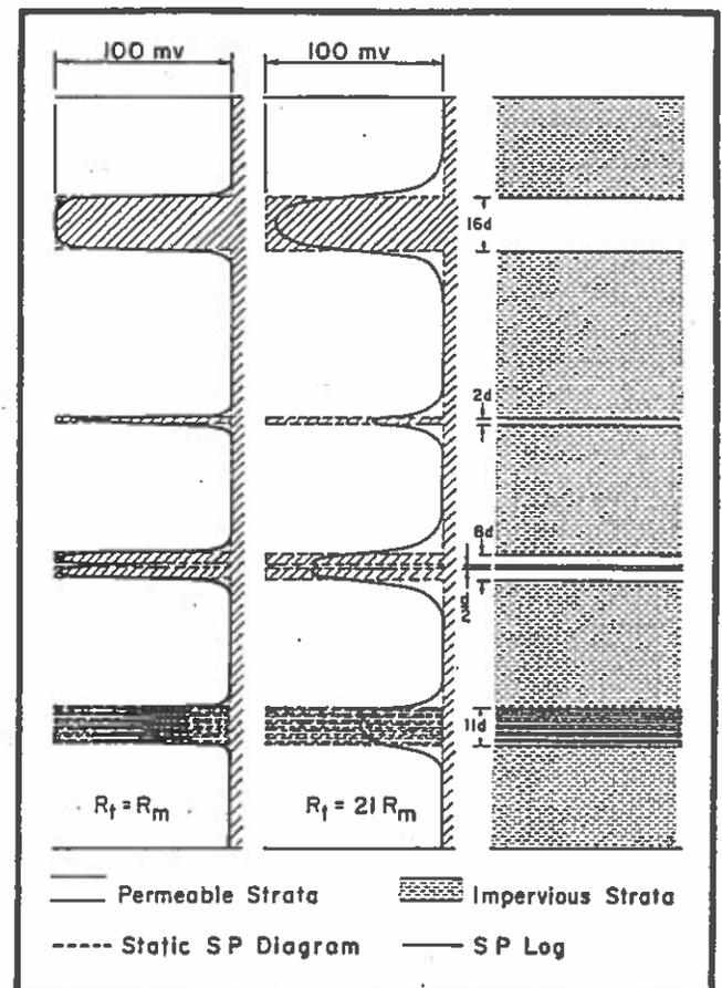
Fig. 2-3 — SP curve in beds of different thickness for  $R_s = R_m$  (left) and  $R_s = 21 R_m$  (center).
