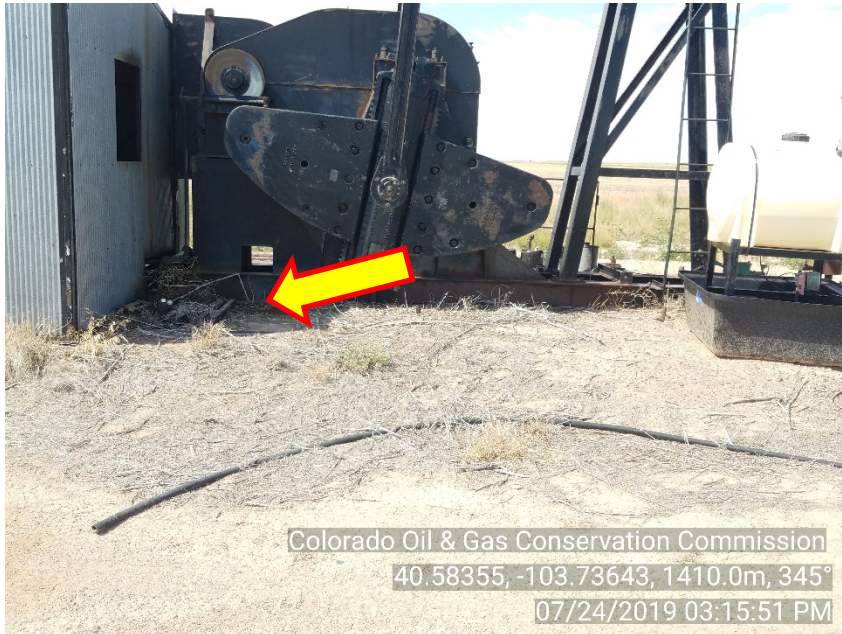
Photo #3 Henderson 1 Pumpjack - South side Stained soil Unused Equipment – plastic pipe Incomplete pumpjack safety guard
