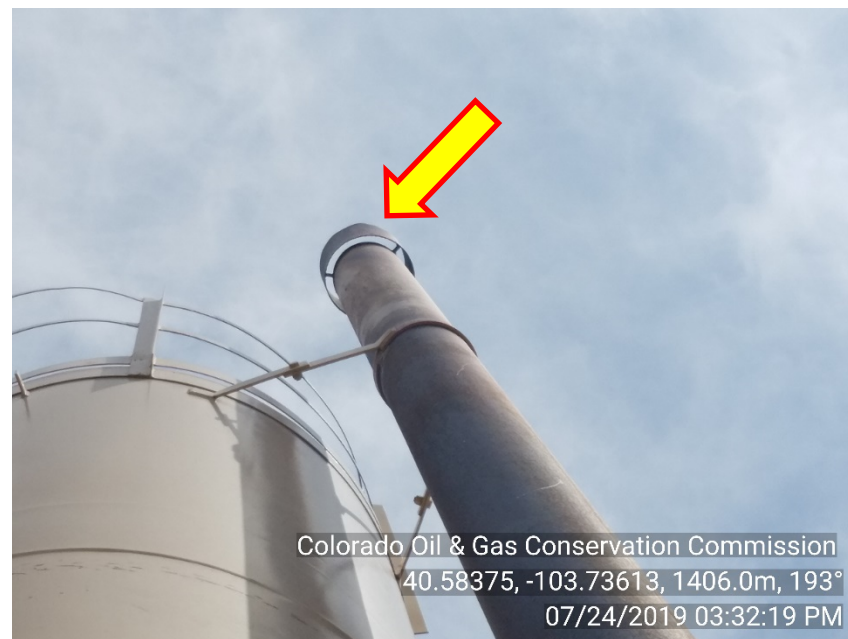
Photo #22 Henderson 1 West treater Bird protection device NOT on stack
