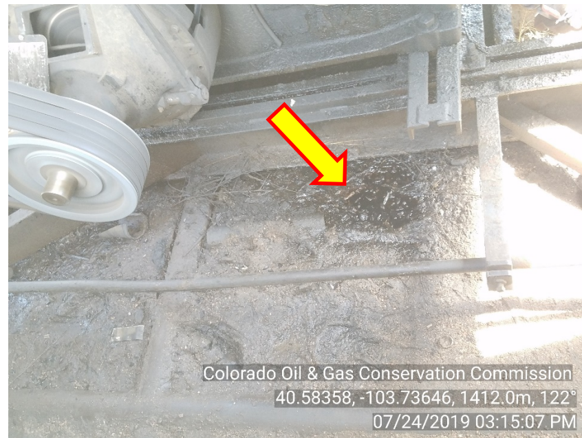
Photo #6 Henderson 1 Engine shed Stained soil - Inside
