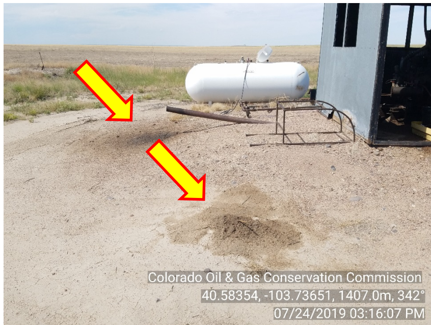
Photo #5 Henderson 1 Engine shed West side Stained soil
