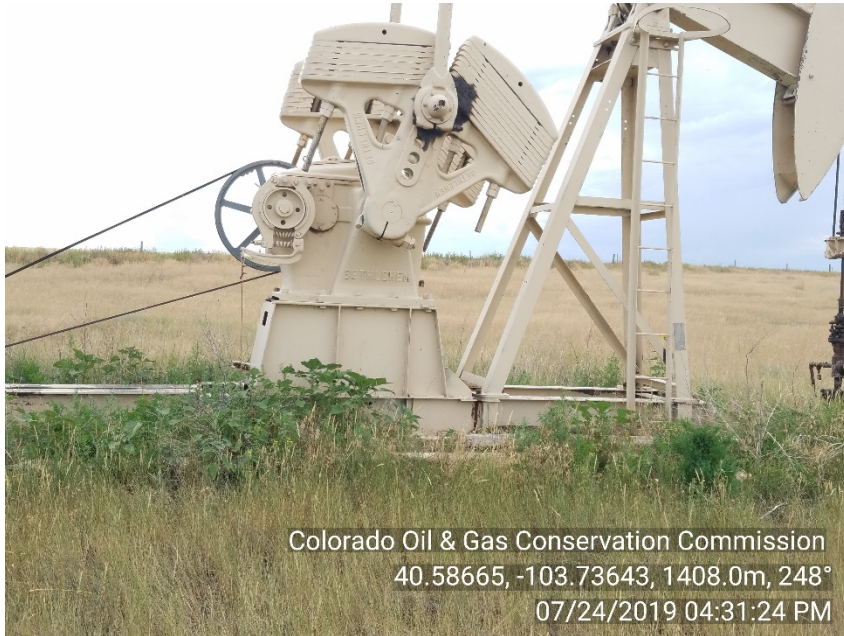
Photo #1 Henderson 2 (05-123-07007) Wellsite Shut-In | SI NO well sign posted No pumpjack safety guard Weeds
