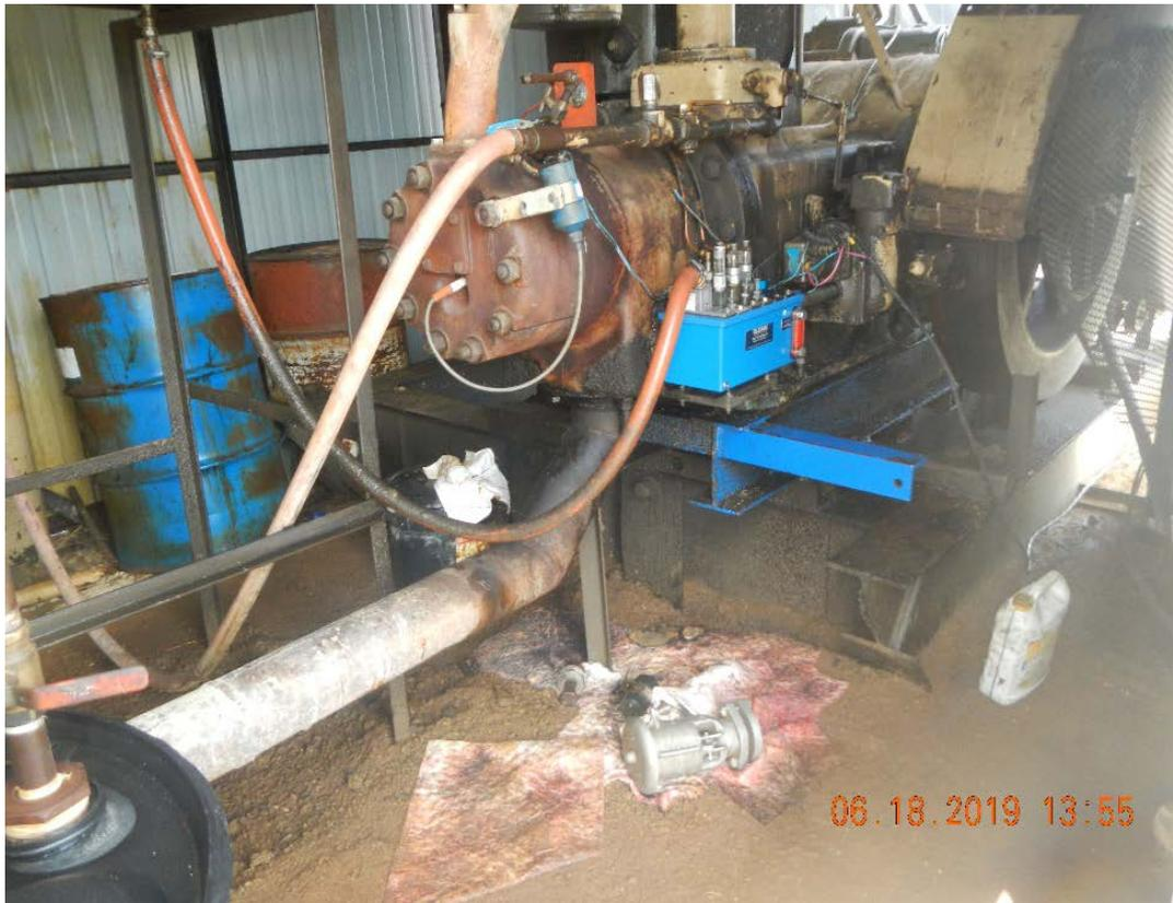
Ptasynski pumpjack motor; oil soil, leaky motor housing.
