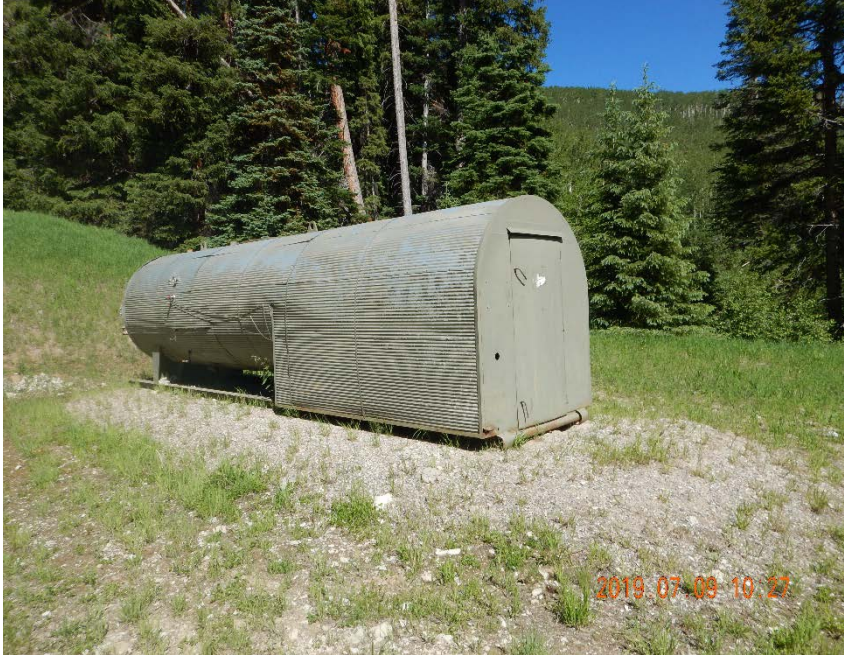
Photo #17 – North unused horizontal treater/separator in Former Tank Battery area.
