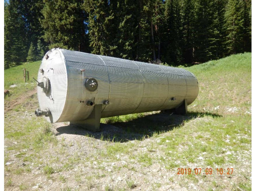
Photo #18 - South unused horizontal treater/separator in Former Tank Battery area.
