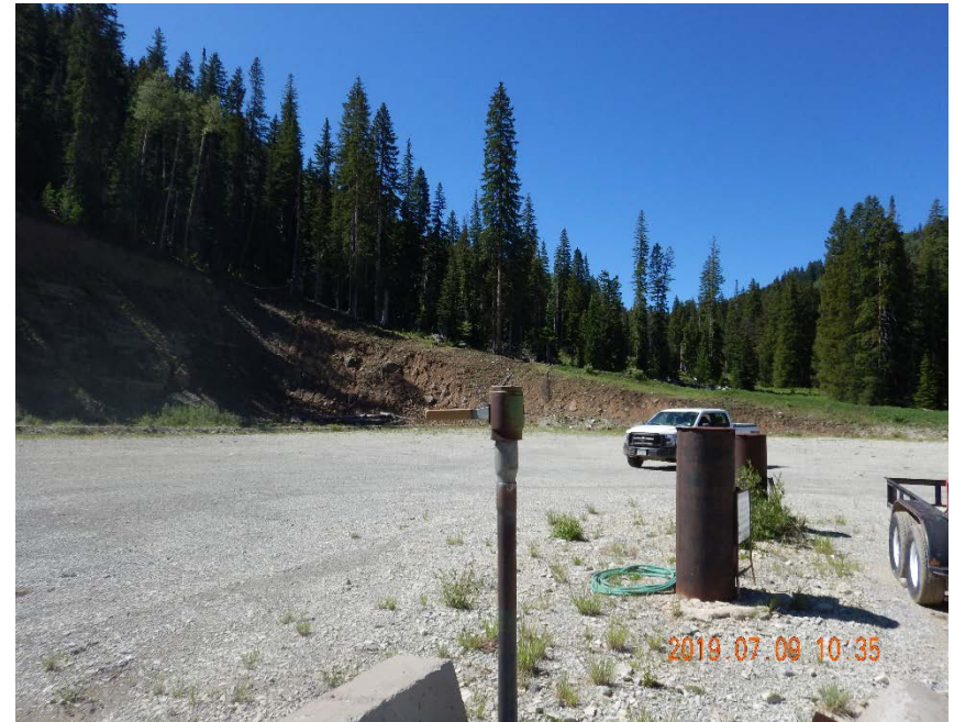
Photo #4 – Uncapped, unmarked flowline riser attached to TPR 132-36.
