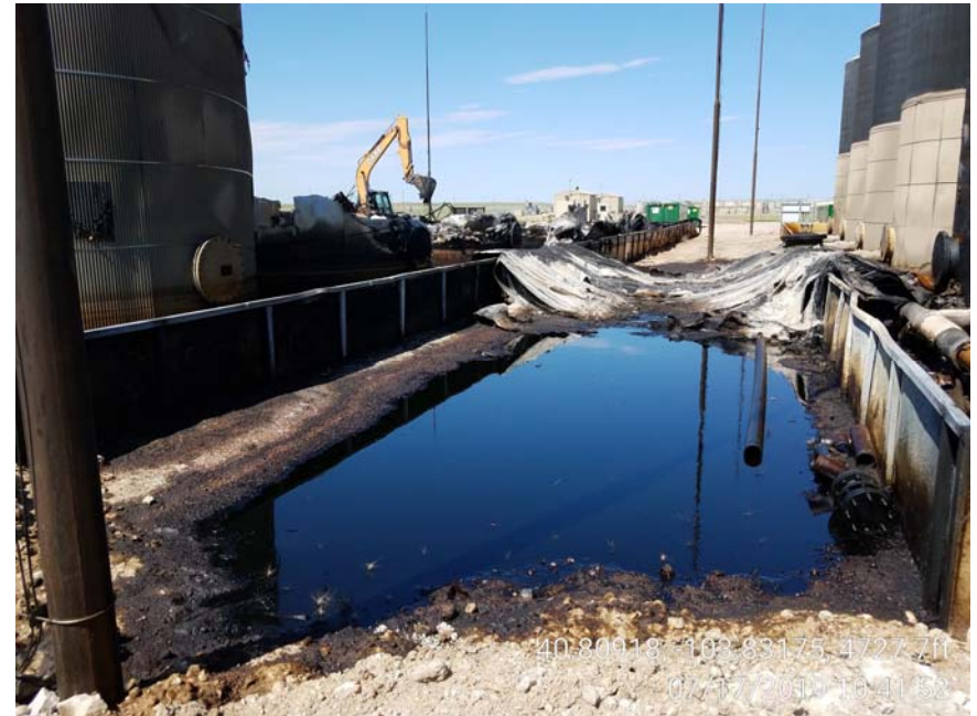
Photo 12 – Standing crude oil near damaged tank battery.
