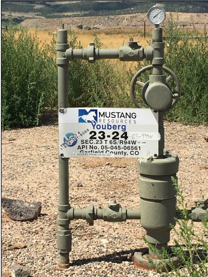
Wellhead and location information
