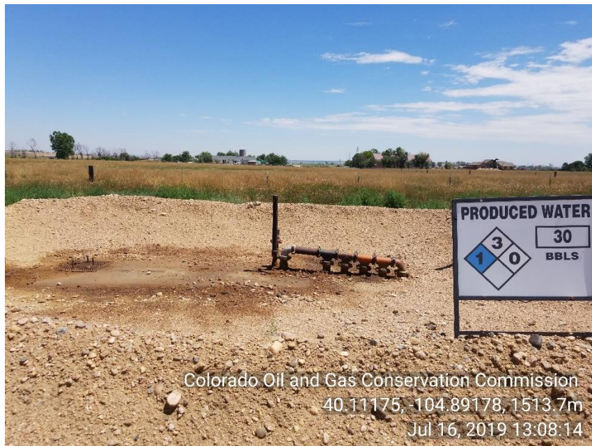
Photo 9 Produced water tank. Appears tank overflowed inside containment. Spill
