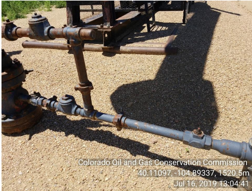
Photo 3 flow lines from Well head are closed
