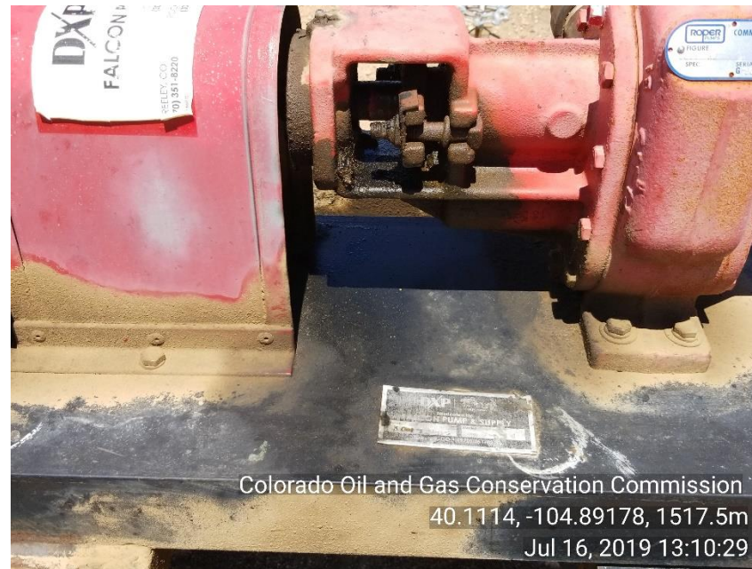
Photo 16 Mechanical issue: recirc pump appears to be leaking.
