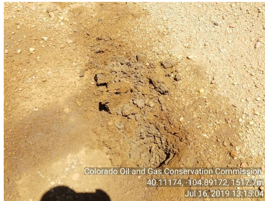
Photo 10 Dug down approx.. 1 ft next to produced water tank ground saturated with what appears to be E&P substance.
