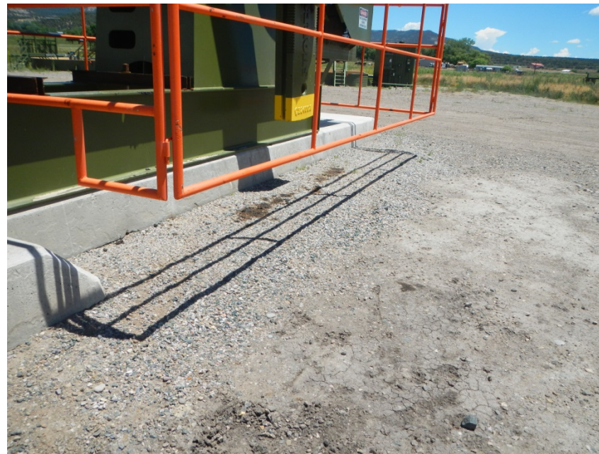
Housekeeping – lube oil accumulating on ground
