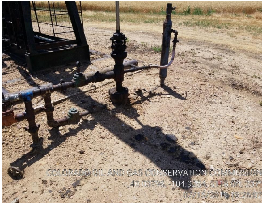
Pic 3 stained soil/possible leak at wellhead
