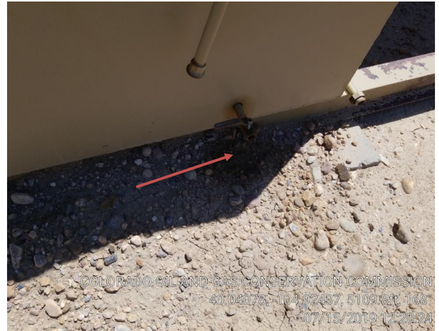
Pic 6 stained soil/possible leak outside of separator
