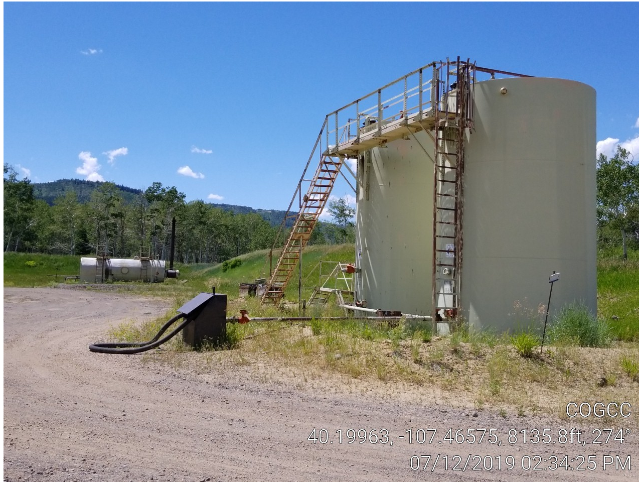
Photo 2. Tank battery & treater.
