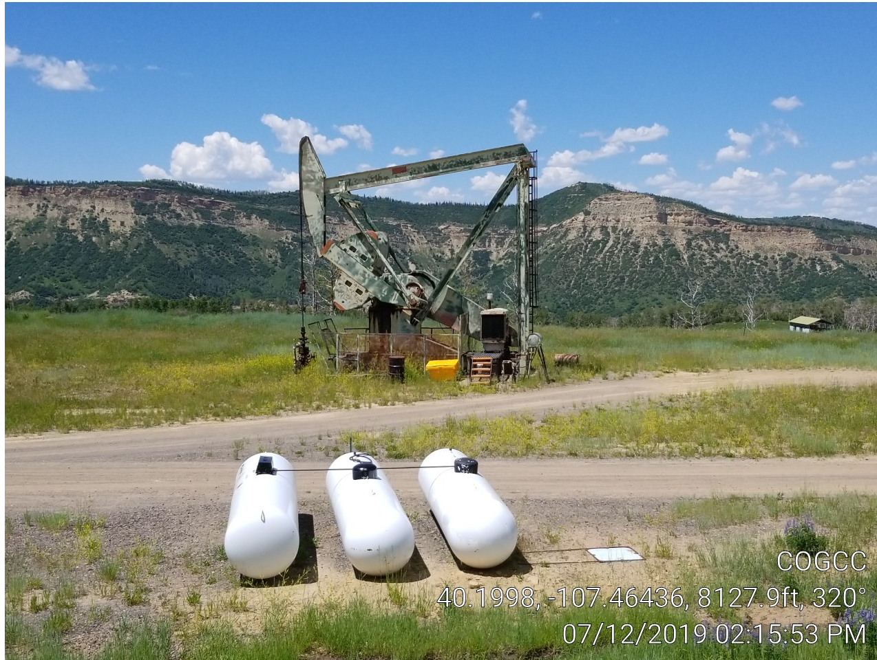
Photo 1. Pump jack & propane tanks.
