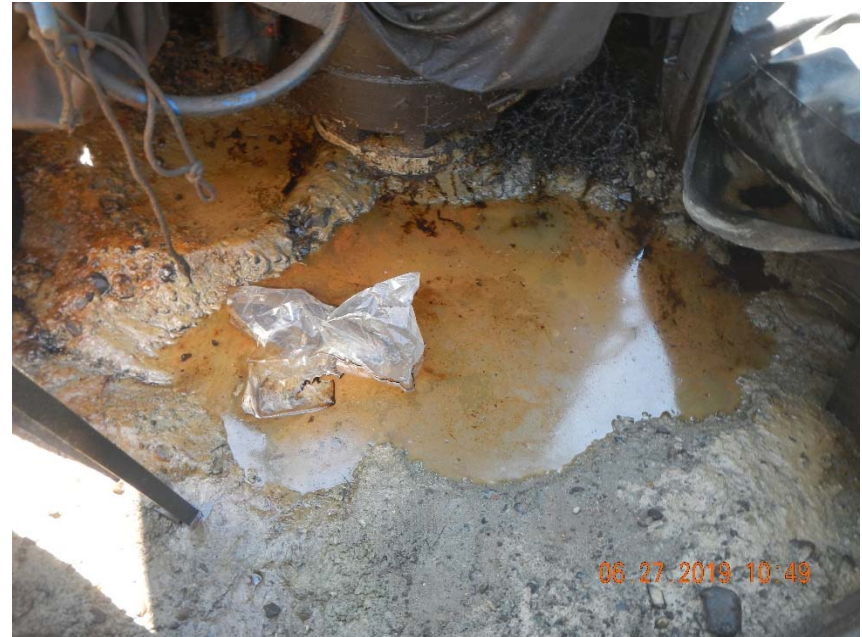
Photo 4. Close up of photo 3, free product and fluid in cellar, debris in/around cellar.
