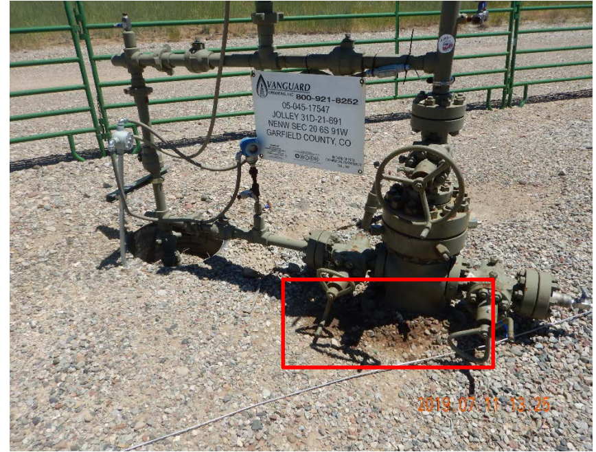
Photo #6 - Jolley 31D-21-691 wellhead. Note localized accumulation of oil-stained material beneath wellhead.
