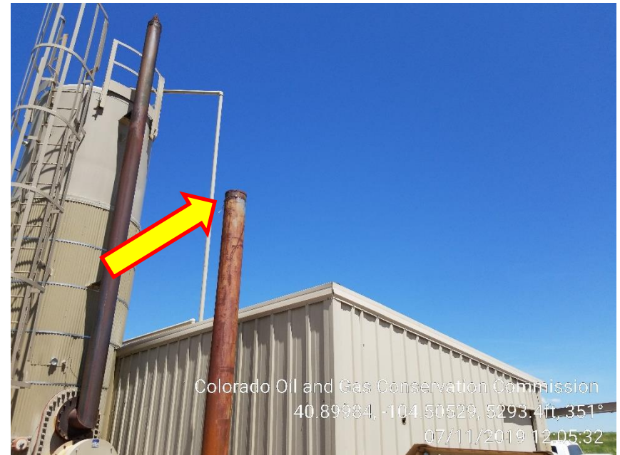
Photo 6 – Glycol unit missing bird protector
