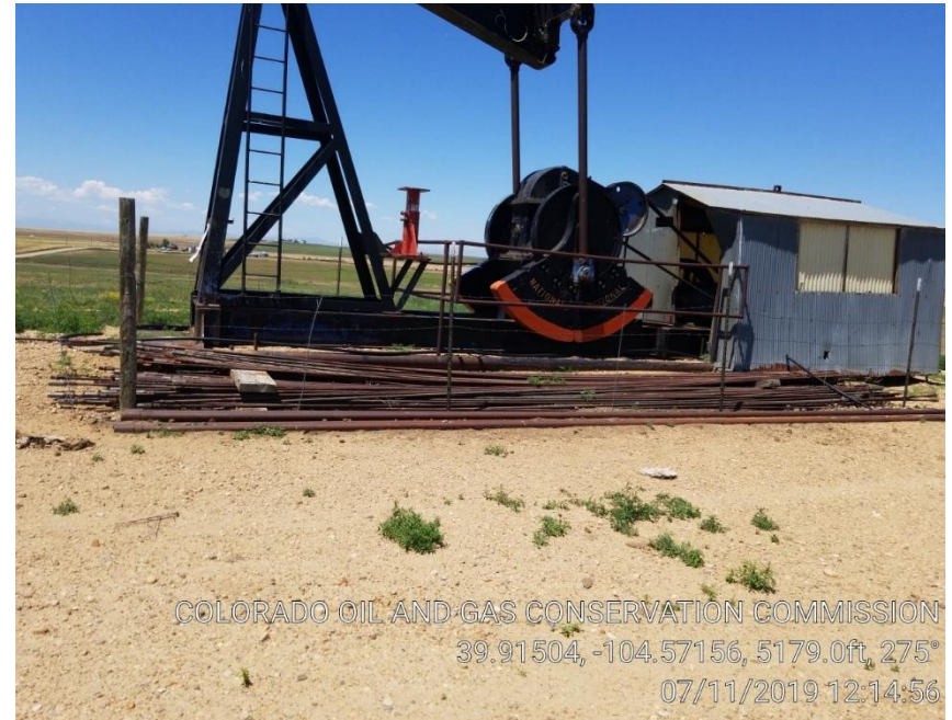
Pic 2 unused equipment sucker rods and tubing
