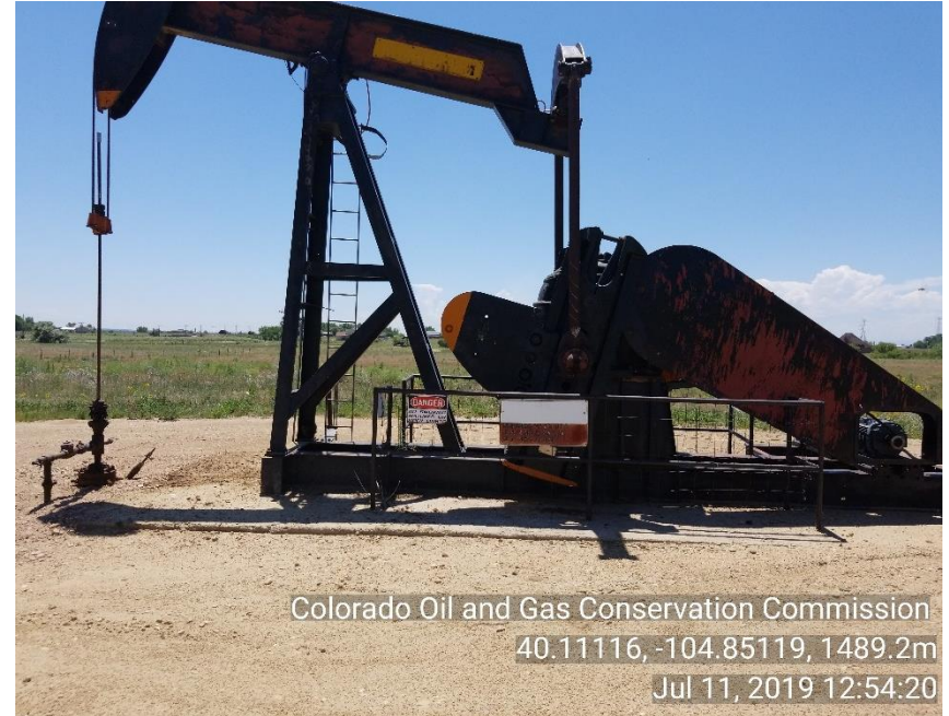
Photo 2 Well Head sign faded not legible.
