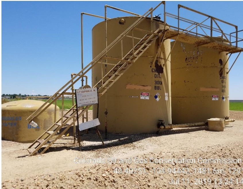
Photo 1: Tank Battery
