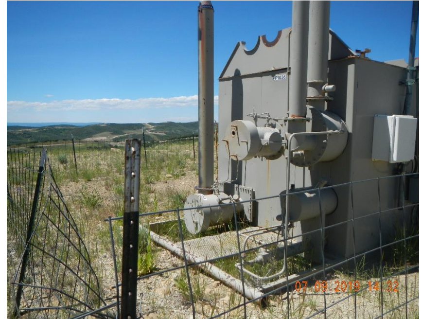
Photo 4 Weeds around heated separator.
