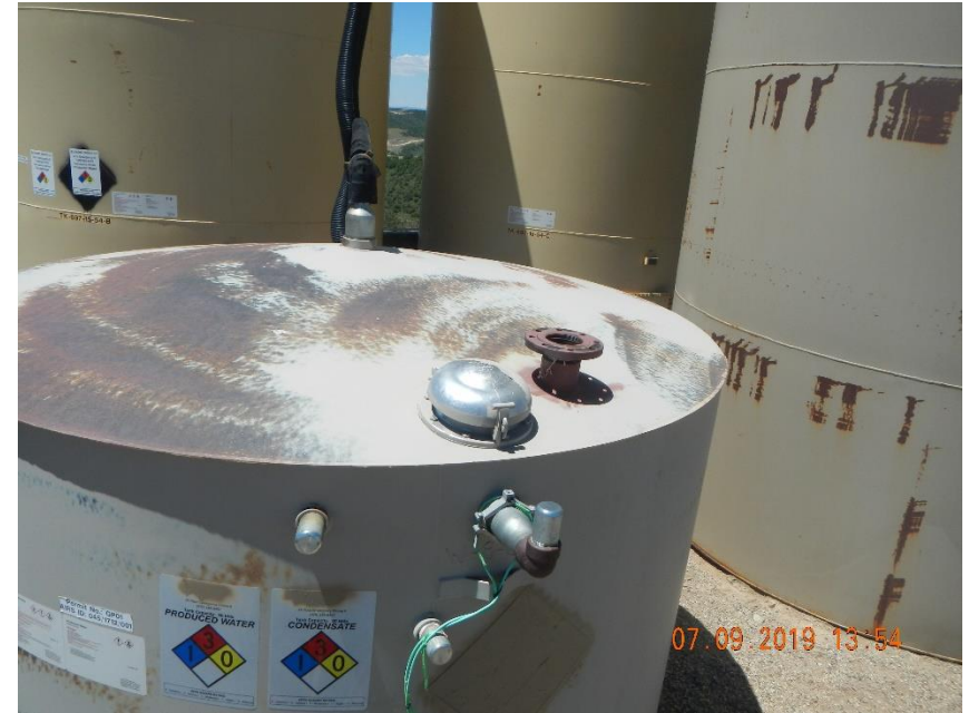
Photo 8 Open port on top of tank.
