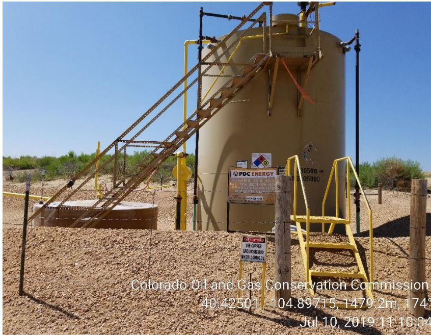
Photo 1: Centralized Tank Battery
