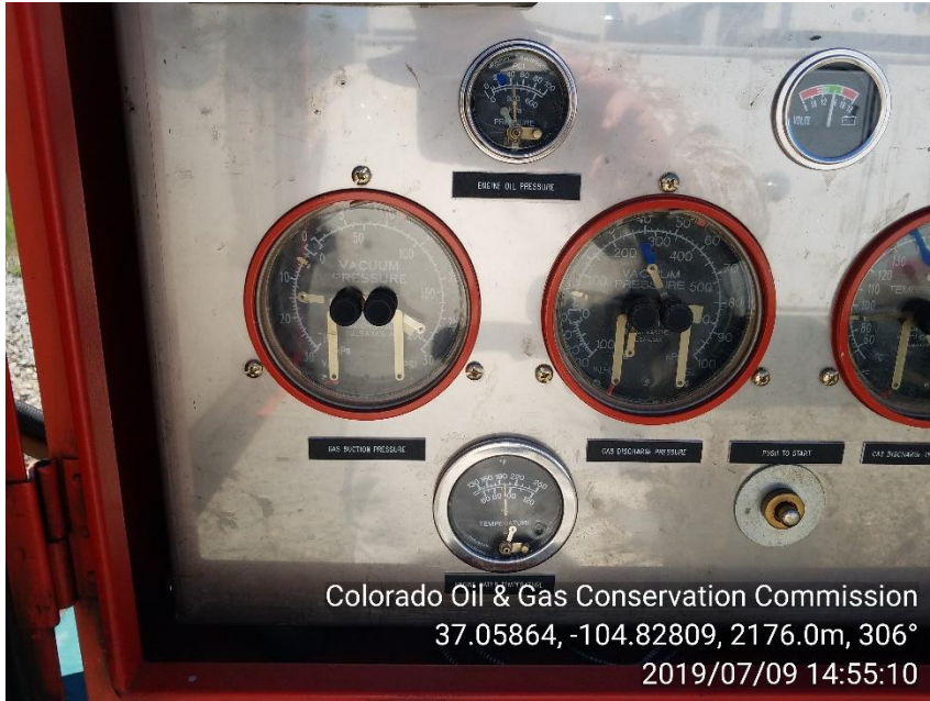
PHOTO 3: Vacuum pump observed on well without COGCC approval. Provide COGCC with documentation showing approval of use of vacuum pump. Ca date 7/24/19
