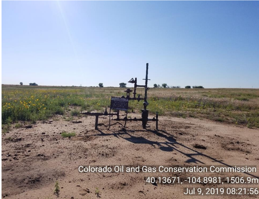
Photo 1 WH and WH sign. Sign needs to be replaced due to having bullet holes. At time of inspection WH appears to be leaking by top of casing.
