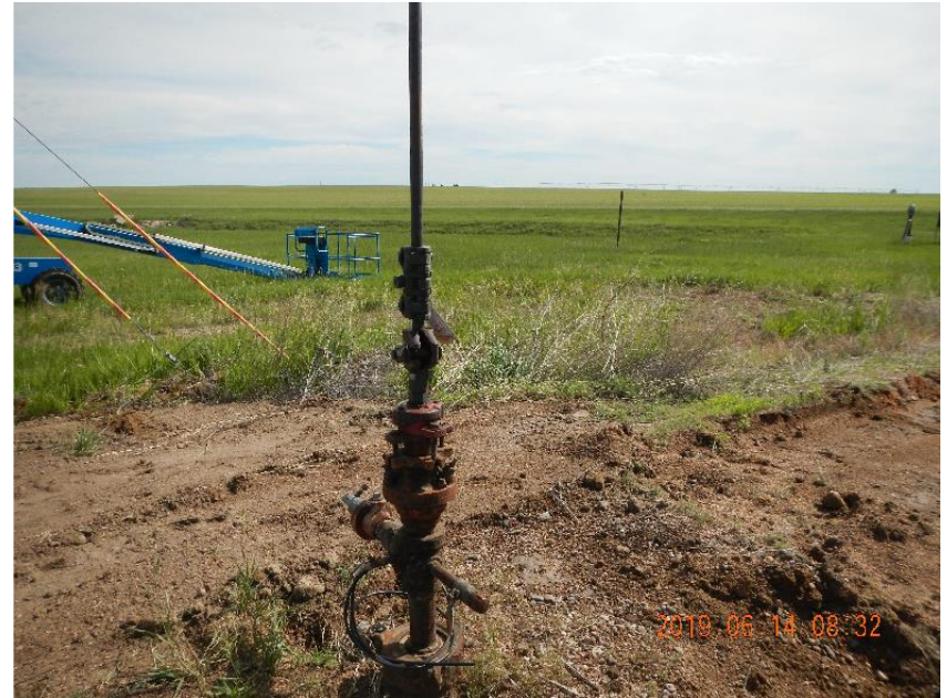
Photo 6: Wellhead with power box and pole removed.
